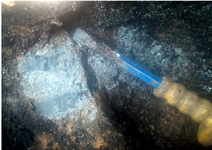
Picture 6: Details of sample 119390464. Abundant Po mineralization from L'Ours occurrence inside an exhalite horizon.
