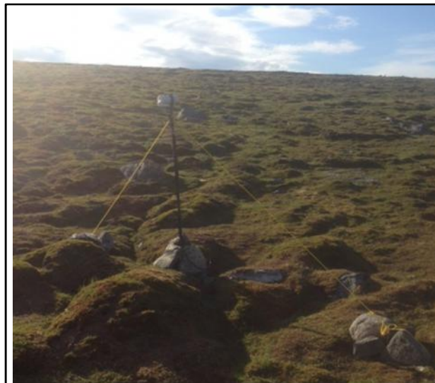
Figure 5. base station magnetometer
