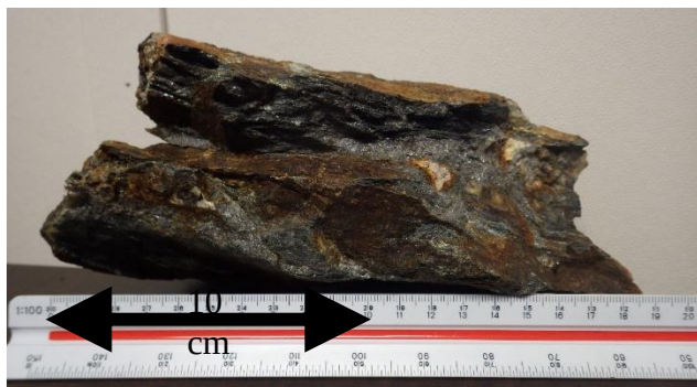
Picture 3b) Sheared basalt with disseminated and massive arsenopyrite
