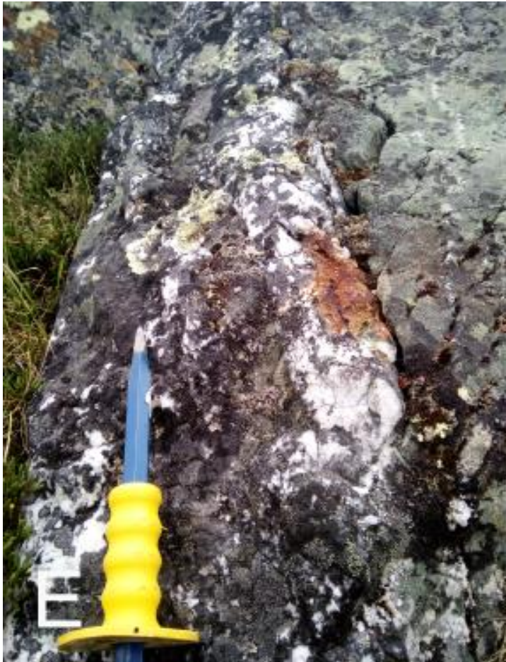
Picture 6: Mineralized quartz vein in ABG Zone, sample P137327 returned 1.23% Cu
