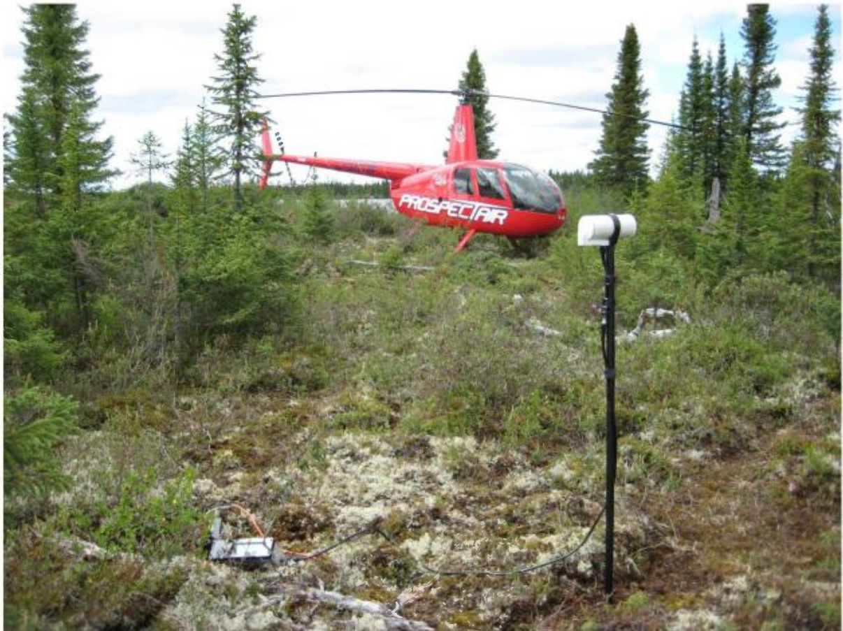
Figure 7: Example of a magnetic base station setup
