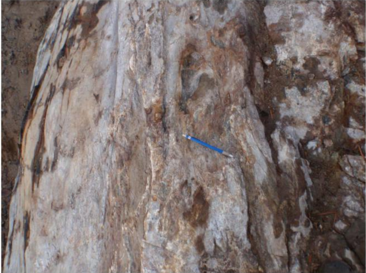
Photo 5 - Interceptor gold-bearing quartz vein, showing laminar structure with folded fragments of altered greywacke. Pencil for scale
