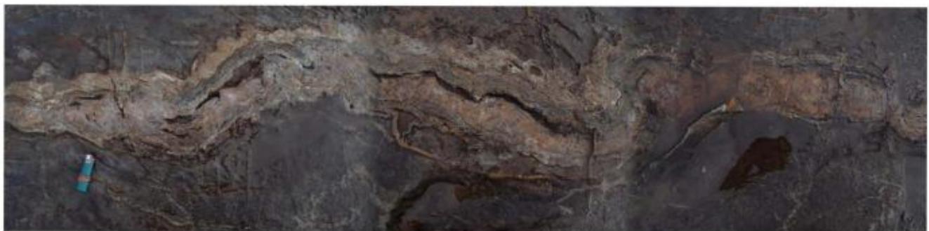
Photo 6 - Panoramic view of gold-bearing laminated quartz vein exposed in the extension of WB2012TR015
