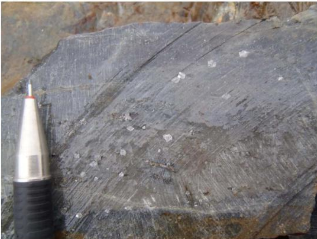
Photo 3: WB2012TR011-R2 at 1.8 meters: 5% pervasive hypidiomorphic arsenopyrite with 2% pyrrhotite and pyrite millimetric stingers in the footwall of the Mustang vein.
