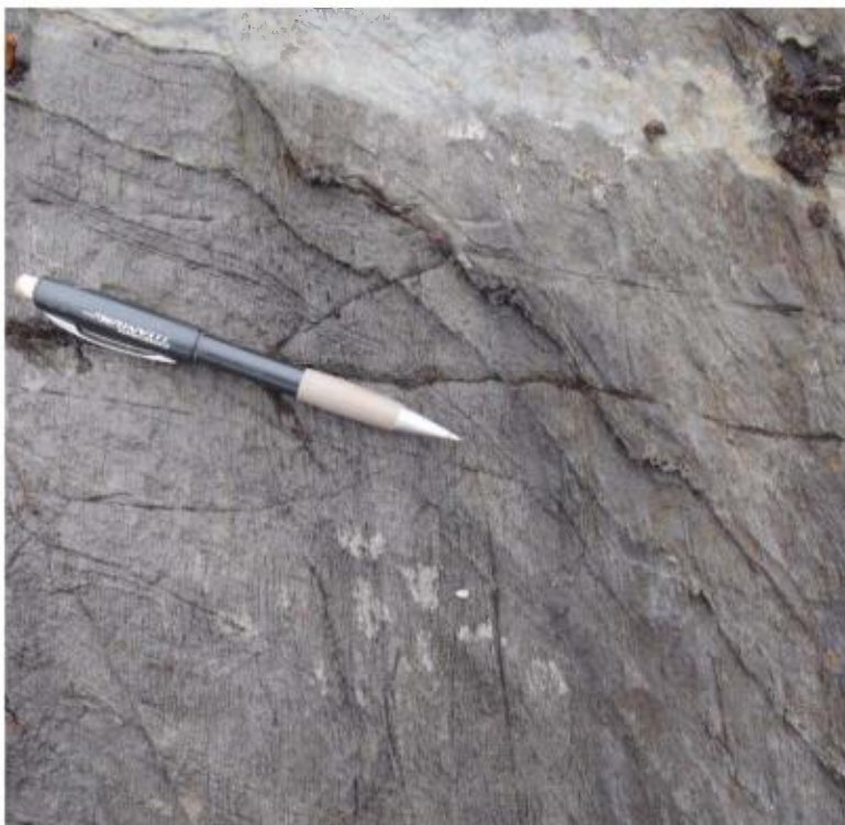
Photo 11: WB2012TR009 : Relationship between the folded bedding (S0) and the main schistosity N250. The early quartz veinlets are also folded and follow the bedding.
