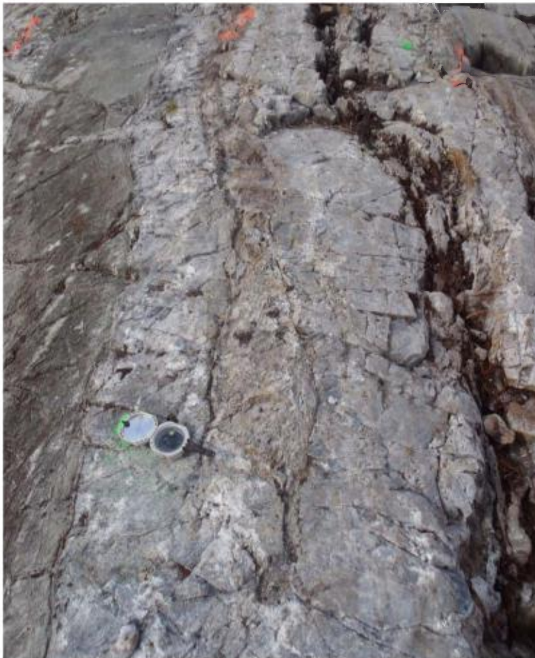
Photo 14 : WB2012TR011 : Mustang vein which has a thickness of 1.5 meters. It is in contact with gabbro (south) and altered wacke (north). The vein has incorporated a fragment of altered wacke that is affected by the main schistosity. Some extensional veins have also developed.
