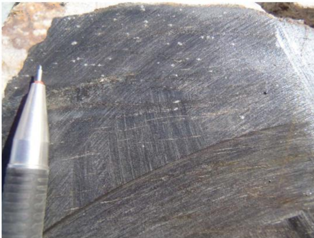
Photo 4: WB2012TR011-R9 located between 0 and 1.70 meters: Pressure shadows created by the granular grains of arsenopyrite (3%) are occupied by pyrrhotite stringers (4%).
