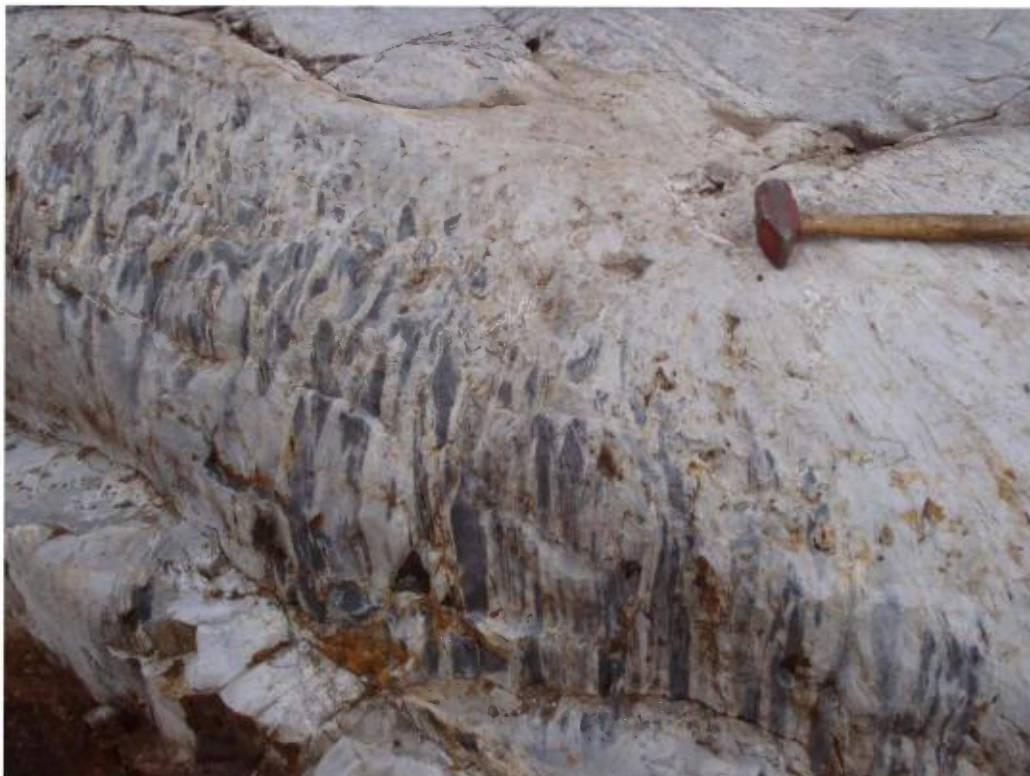
Photo 16: WB2012TR011 : Wacke strongly altered (silica, feldspar, sericite, chlorite) with a fragmentary-banded texture typical of the footwall of the gold-bearing Mustang vein.
