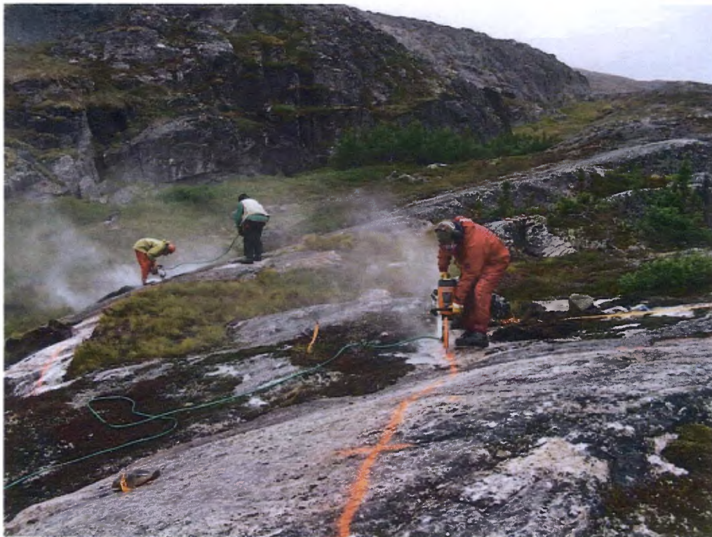
Channel sampling on the Jonas Centre Zone, September, 2009 – looking southward. Note the shallow dip of the gneissosity to the east.
