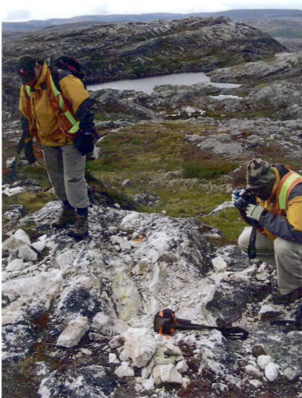
Jonas Upper Zone mineralized pegmatite with yellow uranophane visible in foreground. Looking WNW across Jonas Centre Zone (not visible - below hillside) towards Jonas West on right flank of hill summit in middle distance.
