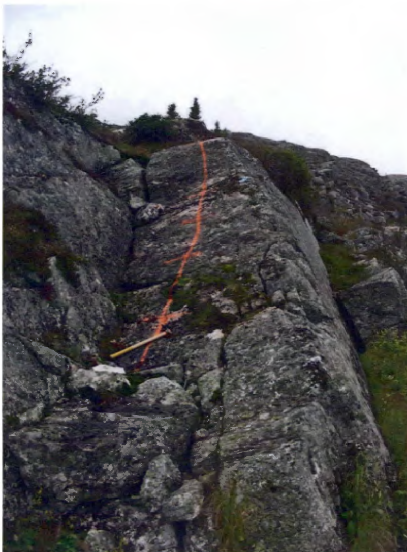
The “Jonas 3.3” fracture-controlled uranium occurrence channel line looking west. Note the steeply north-dipping block fault scarps.
