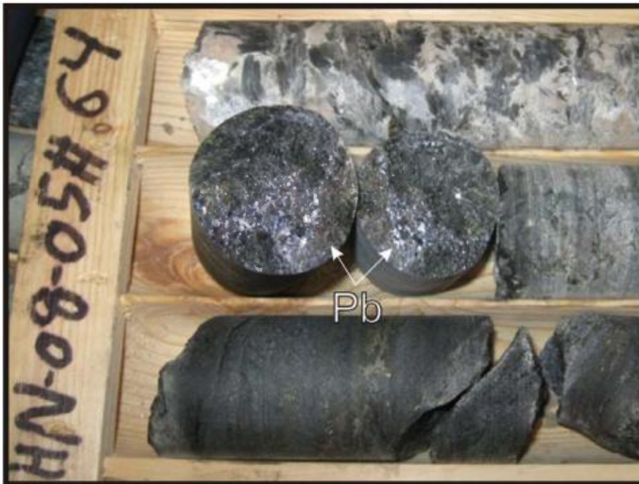
Figure 9-5. Photograph of drill core from DDH HN-08-05 (294.1-295 m) showing galena mineralization in the gabbro. Drill core diameter is 47.6 mm.
