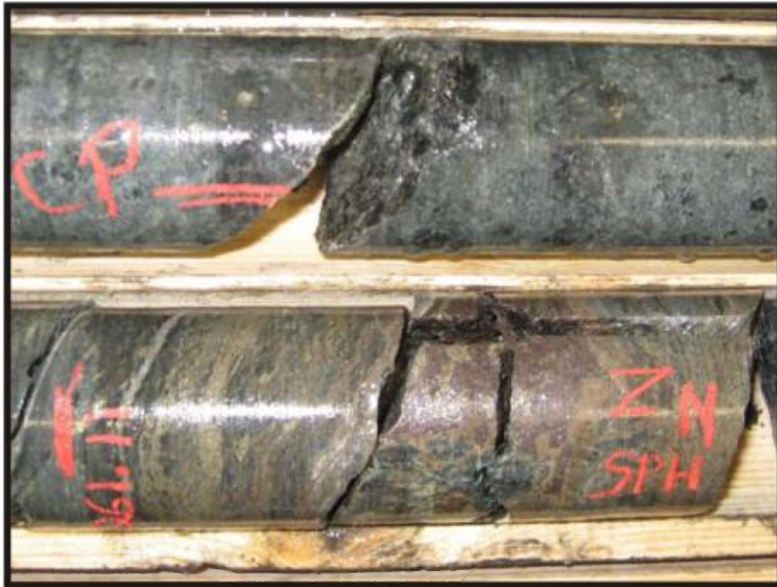
Figure 9-4. Photograph of drill core from DDH HN-08-17 (261.11-261.25 m) showing sphalerite mineralization in the gabbro. Drill core diameter is 47.6 mm.
