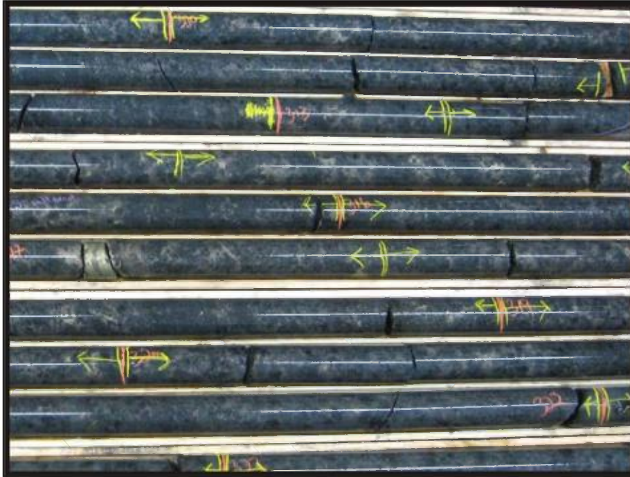
Figure 9-2. Photograph of drill core from DDH HN-08-53 (260.02–332.20 m) consisting of disseminated to blebby pyrrhotite, pyrite and chalcopyrite in the medium- to coarse-grained gabbro near the contact with the metasedimentary rocks. Drill core diameter is 47.6 mm.
