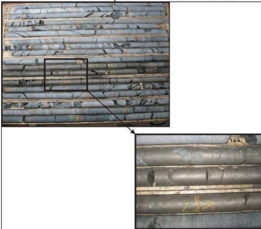
Figure 9-3. Photograph of drill core from DDH HN-08-07 (102.71-107.00 m) showing large blebs of pyrrhotite, pyrite and chalcopyrite and massive sulfide in a shear zone at the contact between gabbro and metasedimentary rocks. Drill core diameter is 47.6 mm.
