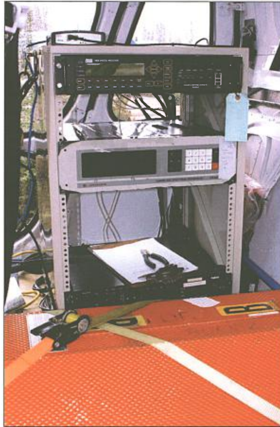
Figure 7: Chaîne d'acquisition Fugro HeliDAS Integreted
