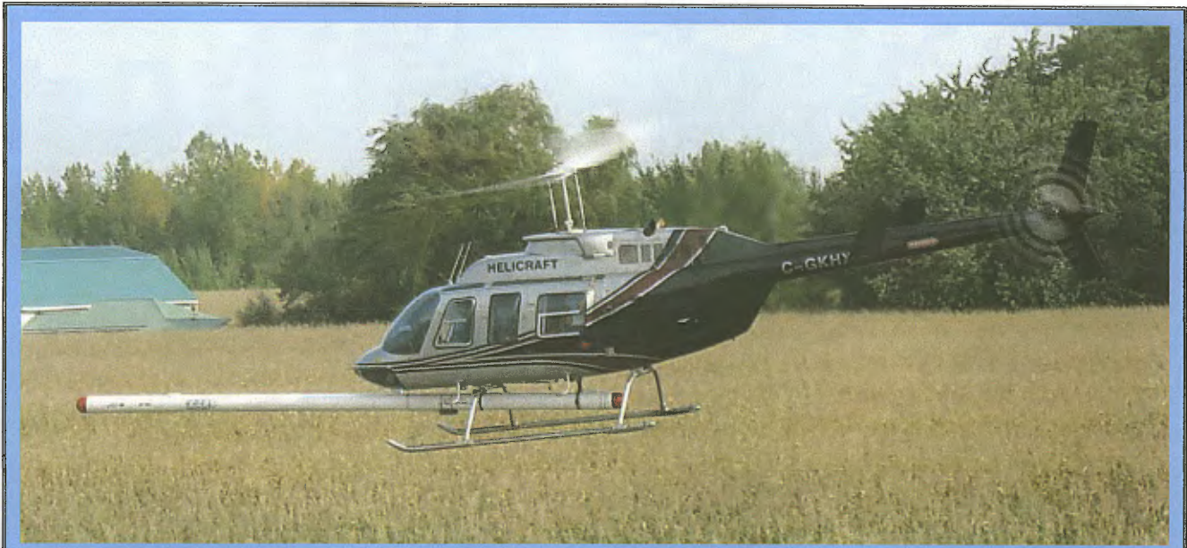
Figure 2: Stinger Installation of the Magnetometer
