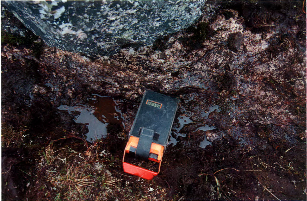
Figure 12: Urtec UG-135 #3 with a reading of 10744 cps on a pegmatite. Note shearing evidence in pegmatite.
