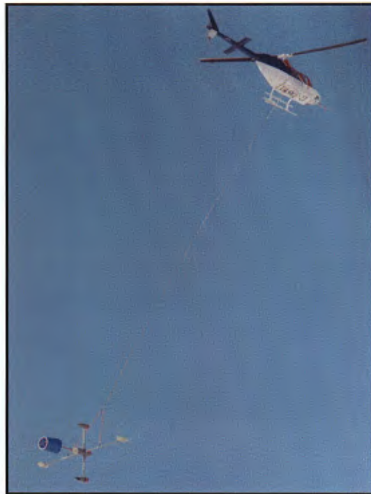
Figure 4 – Helimager™ in flight with a Bell 206-B
