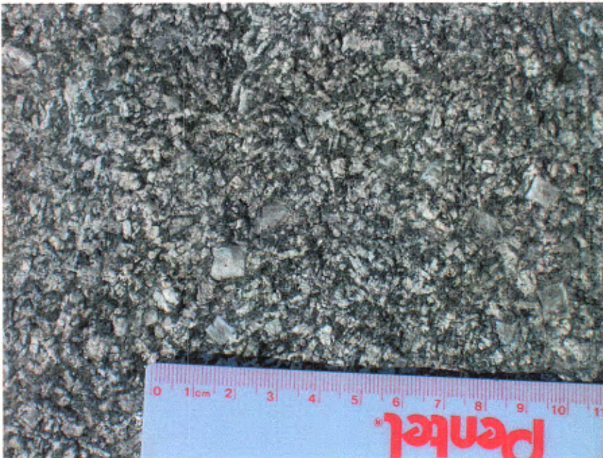
Photo 12: Monzodiorite with euhedral phenocrysts of feldspar and a groundmass of feldspar and pyroxene
