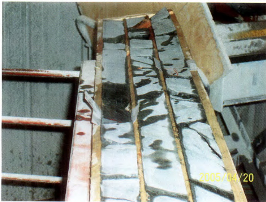
Figure 36: View of a core box with two sampling tags before cutting the core half in 2 quarters.
