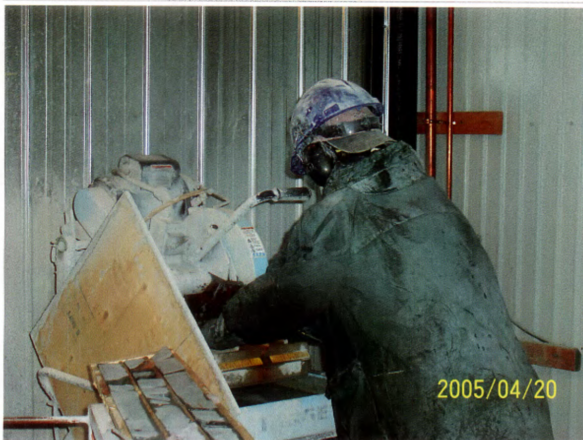
Figure 31: Vior technician cutting the core with the rock saw at Douay facilities
