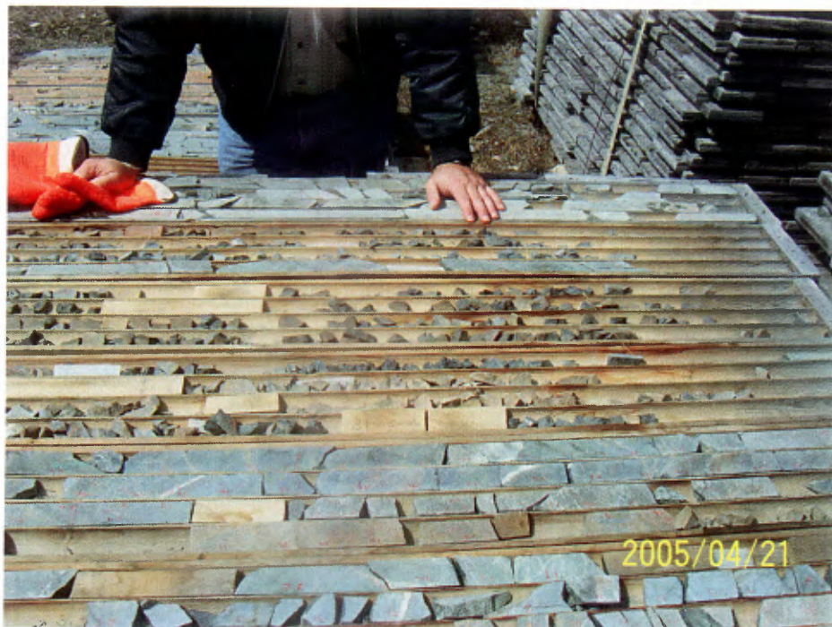
Figure 37: View of the core left in the box after many samplings by Vior's different partners
