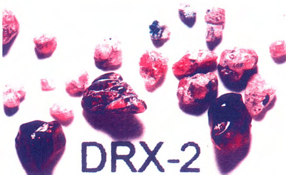
PHOTOGRAPH 2 SAMPLES: DRX- 1 & DRX-2; CAUSTIC FUSION RESIDUE PINK CORUNDUM AND PYROPE GARNET TORNGAT PROJECT, QUEBEC DIAMOND DISCOVERIES INTERNATIONAL
