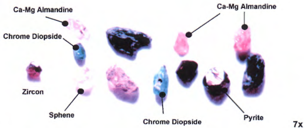
PHOTOGRAPH 5. DDI-3 SERIES SAMPLES CHROME DIOPSIDE, PHLOGOPITE, SPHENE, Ca-Mg ALMANDINE TORNGAT PROJECT, QUEBEC DIAMOND DISCOVERIES INTERNATIONAL
