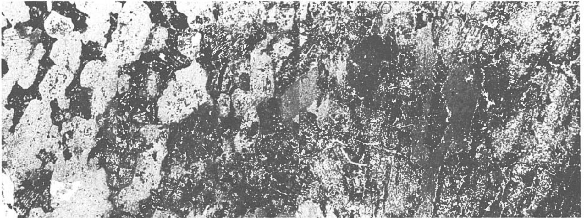
Fig. 54. Photomicrograph across the contact of a metagabbro (right) and magnetite-rich metaferropyroxenite (left) (LZ). The elongation of the plagioclase and pyroxene grains in the gabbro is preserved and imparts a distinct igneous lamination to the rock parallel to the layering. Small pyroxene grains are left in the cores of amphiboles at the left side. The Widmanstätten texture of the titaniferous magnetite is also well preserved. The magnetite is partly replaced by chlorite and minor carbonate. The opaque lamellae have a border of very small grains of sphene. Sample 12-283(220). Field is 2.5 cm wide.
