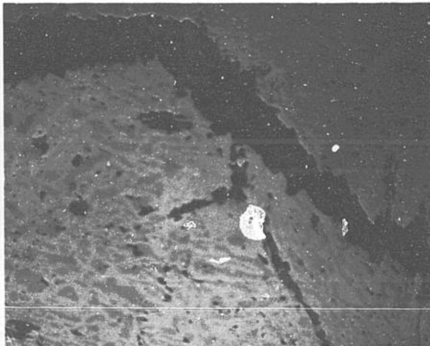
Fig. 146. Photomicrograph of polished section in reflected light. Micrographic intergrowths of ilmenite (dark grey) and titaniferous magnetite (pale grey matrix). From Caty (1970), plate 7A, p.94. Width of field is 0.6 mm.
