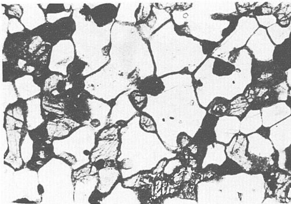
Fig. 72. Photomicrograph of pyroxene ferrodiiorite (FZ). Pyroxene is fresh except for a very narrow rim of chlorite. White is fresh plagioclase. Field: 2.8 mm. Sample B-70-62. from Baskin(1975) fig. 17, p. 42.
