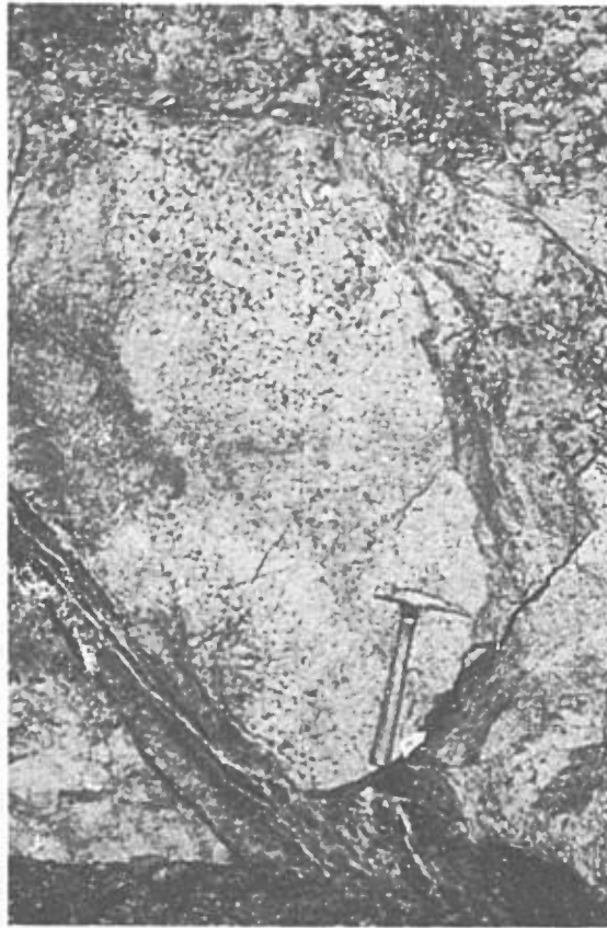
Fig. 130. Meta-anorthosite and gabbroic meta-anorthosite (AZ) cut by intense shear on the left and by many incipient shears at top and right central part of the photograph. Note the good preservation of the cumulus-intercumulus texture in the unaltered (but metamorphosed) block of gabbroic anorthosite. Underground at Jaculet mine.
