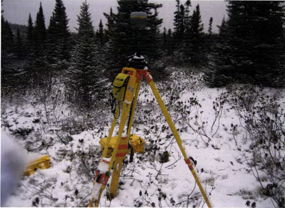
Figure 6. Station de base GPS
