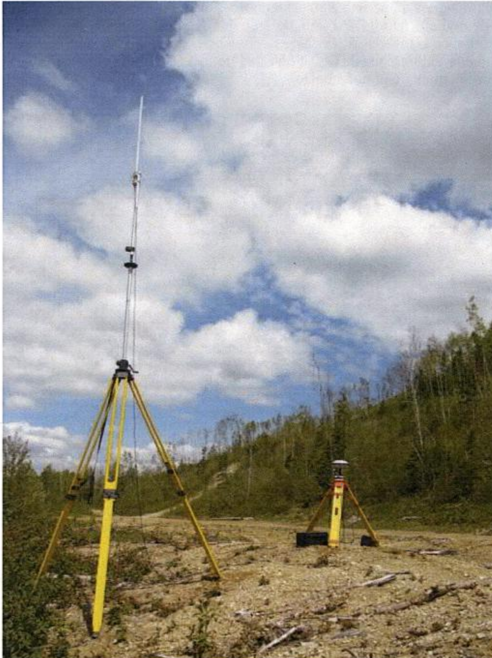
Figure 6. Figure montrant la station de base RTK ProMark 500 de Magellan et la station émettrice Pacific Crest.
